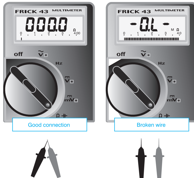
Figure 4.7 Sample meter readings
