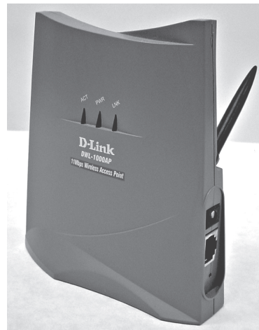
Figure 13.25 A D-Link access point
