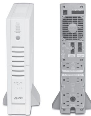
Figure 4.19 Front and back of a UPS
