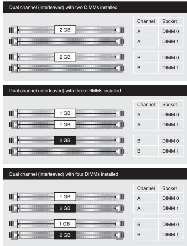
Figure 6.6 The total capacity of the memory module installed in Channel A should match the total capacity in Channel B.
